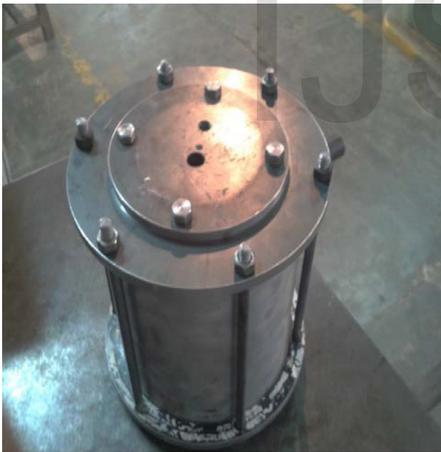
Fig 1: A segmental view of combustion chamber before assembly
