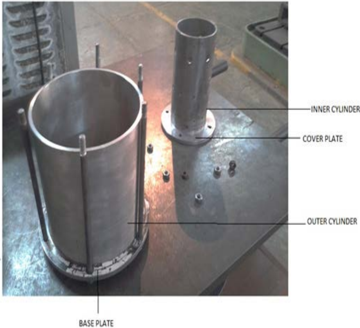
Fig 1: A segmental view of combustion chamber before assembly
