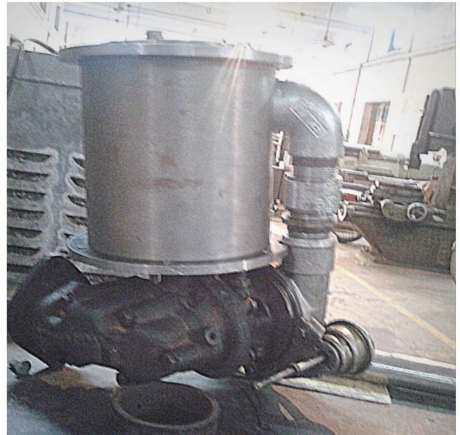
Fig 3: Typical turbojet assembly before testing
